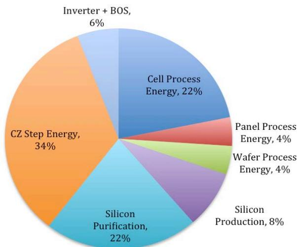
**Figure 2.** The distribution of embodied energy requirements for mc-Si PV [8].
