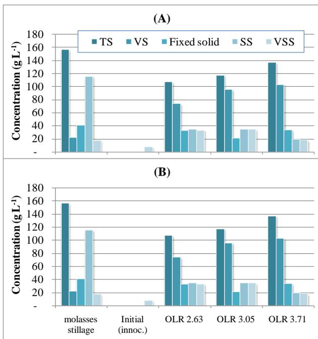
**Figure 3.** Solid concentrations in LM1 (A) and LM2 (B) plotted with OLRs during start up.
