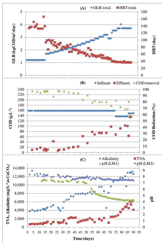
**Figure 1.** Variation of performance parameters with operating time of the two phase semi-CSTR: (A) COD concentration and COD removal efficiency; (B) OLR and HRT; (C) Alkalinity, TVA and pH.
