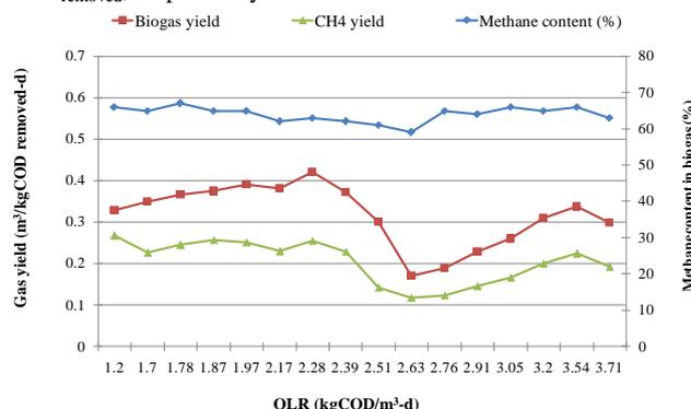
**Figure 2.** Specific biogas and methane yields and methane content in biogas plotted with OLRs during start up.
