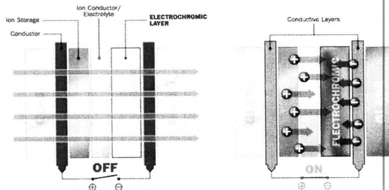
**Figure 1** Multilayer of electrochromic windows [3]
